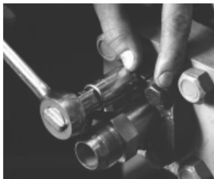
3. Lay the hose assembly into routing position to verify length and correct routing.
