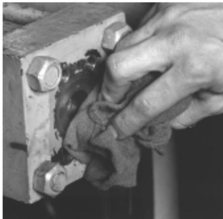
2. Install adaptors into ports (if used). Tighten to manufacturer's recommended torque settings.
