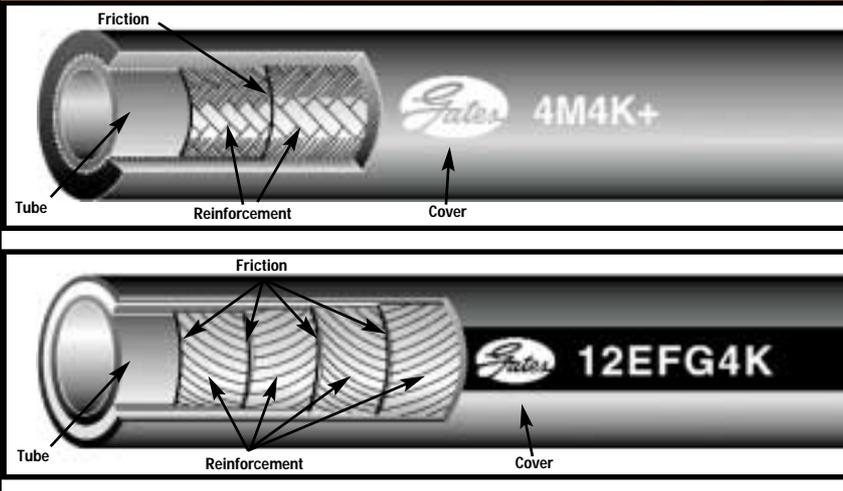
ABOVE AND TOP: Gates' 12EFG4K four-layer spiral hose construction and the 4M4K+ two-layer wire braid hose construction
