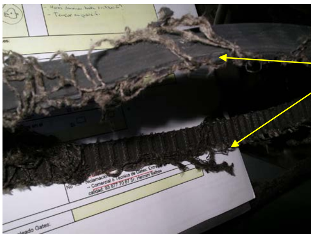
Fig. 2 Typical wear pattern on the side of the belt
