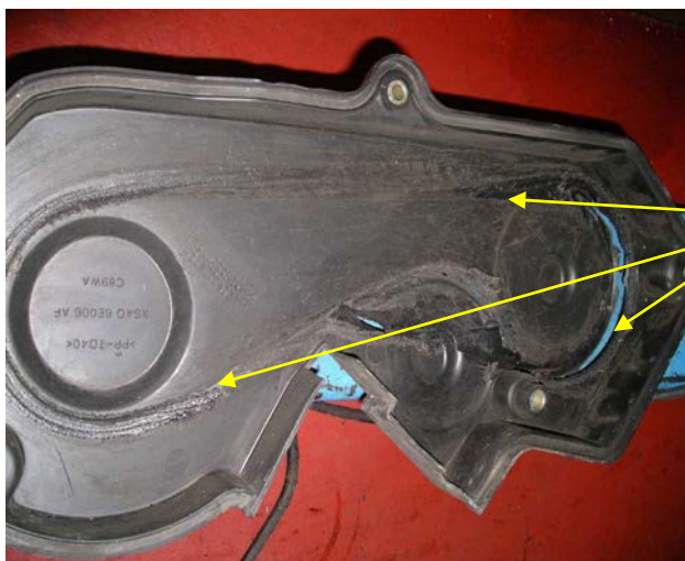
Fig. 3 Signs of serious wear on inside of the cover due to contact with the side of the belt
