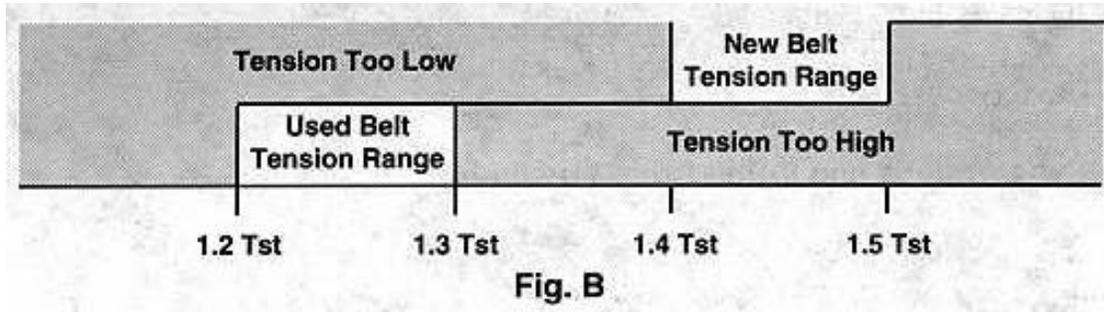
It has always been recognized that we must give the user some tolerance on tension (since it is difficult to install to an exact value), so we have used the idea of a range. The closer a belt drive can be installed to the ideal 1.0 tension value, the lower the stress on all drive components.
