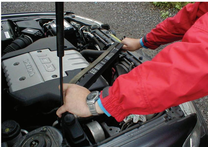
about a change in belt construction, as well as change in the tooth profile — usually, all in a much tighter space. That is why it's vital that the most recent fitting data is consulted every time. You can never be sure when the procedure was last revised," he adds.
