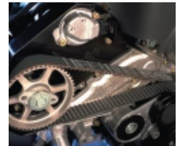
continue to improve resistance to temperature/ wear/ flexibility, as well as increase strength and reliability, the one thing that can't be provided, but which is just as crucial to performance and longevity of the belt, is the correct tension.
