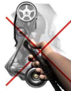
△ Handle the belt with care and store it in its protective box until installation. Never coil, crimp or twist timing belts, as this could damage the tensile cords.
